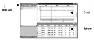
Data Sets Window – Displays how many data sets were loaded and the detail information for each data set (start date, start time, recording rate and data length). Click on any data set to choose the set for graph and tabular window.
